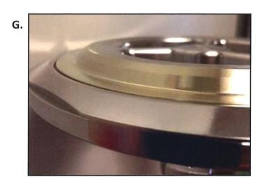
Illustrated here (*picture G.*): This is <u>just the</u> <u>weight of the blade</u> at "0", you can see how it is close to ("flush") the blade is with the depth gauge. This is the reason why a slight amount of pressure is needed during recovery. If slight pressure (*NOT EXTREME*) is applied, it will keep the blade seated properly within the head assembly and in relation to the depth gauge.
