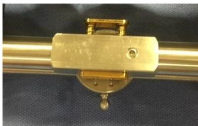
Figure G. Correctly closed push-pull mechanism.
