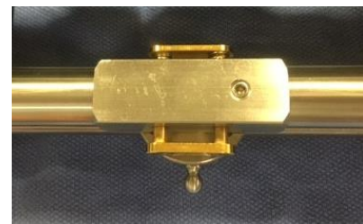
Figure H. Incorrectly closed push-pull mechanism.
