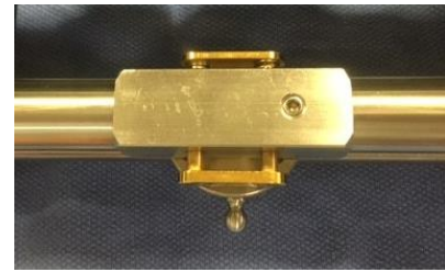
Figure H. Incorrectly closed push-pull mechanism.
