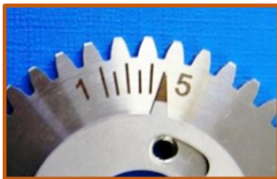
Figure D. Ratio pointer. Shown at 5:1 position.
